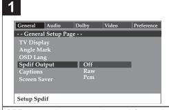
**OFF:** An analog surround sound format is output through the side connectors for two channel audio out or 5.1 channel audio out.
